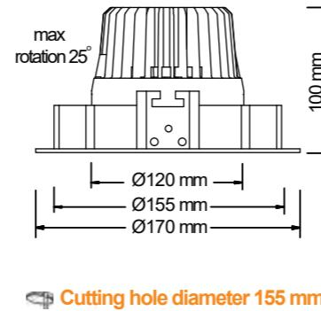
Cutting hole diameter 155 mm
