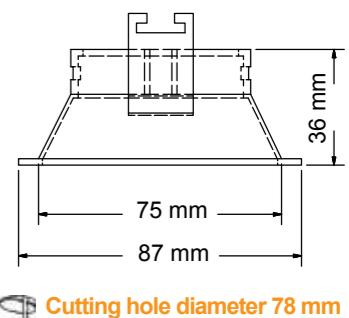
Cutting hole diameter 78 mm
