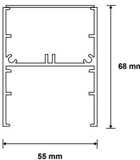
Available in multiple dimensions and finishes (powder coated or anodized).
