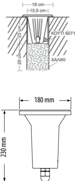
Cutting Hole Diameter 130 mm
