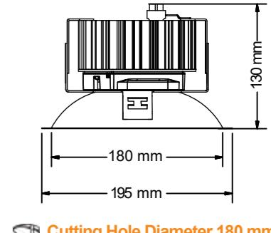
Cutting Hole Diameter 180 mm
