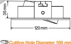
Cutting Hole Diameter 100 mm
