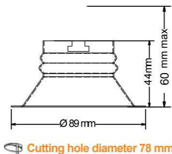
Cutting hole diameter 78 mm
