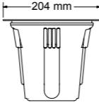
Cutting Hole Diameter 175 mm
