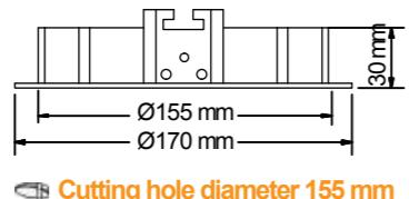
Cutting hole diameter 155 mm
