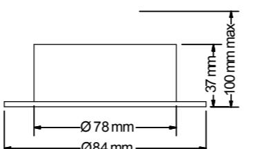
Cutting hole diameter 78 mm
