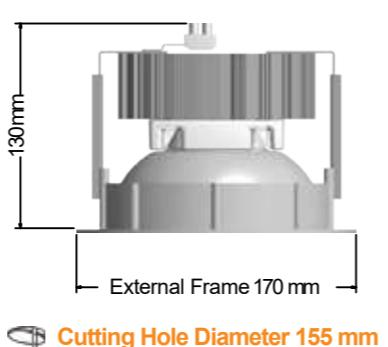
Cutting Hole Diameter 155 mm
